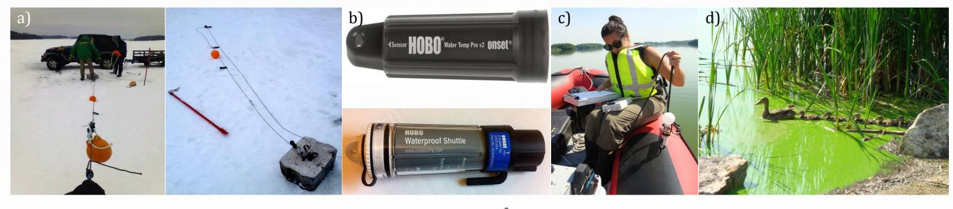
Figure 4. a) The thermistor chain is composed of five temperature HOBO<sup>®</sup> Water Temp Pro v2 u22-001 loggers and was installed when the pond was still frozen. b) HOBO<sup>®</sup> Water Temp Pro v2 u22-001 loggers (top), and HOBO<sup>®</sup> Waterproof Shuttle data downloader (bottom). c) Collecting Photosynthetically Active Radiation (PAR) measurements during weekly sampling. d) Cyanobacteria bloom on June 17, 2014.
