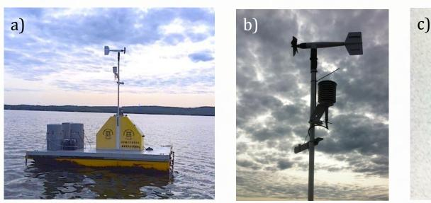
Figure 2. Buoy system on Missisquoi Bay (a) that contains automatic samplers for water, weather station (b) and YSI Sonde (c).
